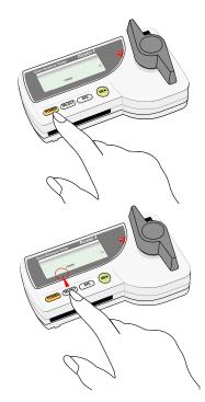
**1** First, confirm that the figures "8 TIMES 88.8%" and several other marks appear when the "POWER" button is pressed with your finger. Should the figures not appear, or batterie mark appear, the batteries are exhausted. Replace all of the batteries with new ones, according to the diagram illustrated in the battery chamber.
