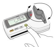
A Rotate the Crushing Handle counterclockwise, and fully insert the Sampling Tray into the Testing Chamber. Fully rotate the Crushing Handle until stop is reached, so that the sample may be well crushed. Press the "MEA" (Measure)button, the most reliable moisture content is then displayed to be read directly without using any conversion tables.
